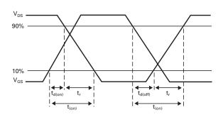
**Switching time waveforms**
