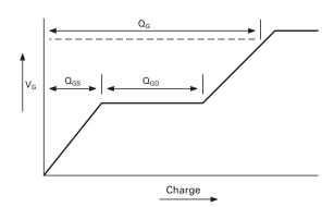
Basic gate charge waveform
