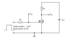
Switching time test circuit
