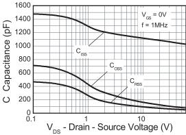
Capacitance v Drain-Source Voltage
