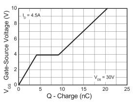
Gate-Source Voltage v Gate Charge
