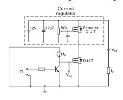
Gate charge test circuit
