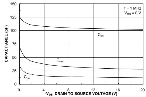
**Figure 8. Capacitance Characteristics.**
