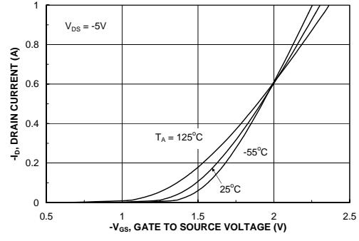
Figure 5. Transfer Characteristics.
