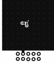
a) 200°C/W when mounted on a 1in<sup>2</sup> pad of 2 oz copper
