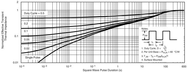
Normalized Thermal Transient Impedance, Junction-to-Ambient
