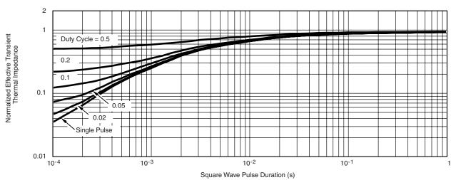
Normalized Thermal Transient Impedance, Junction-to-Case
