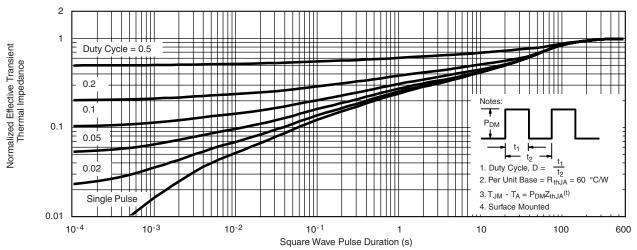
Normalized Thermal Transient Impedance, Junction-to-Ambient
