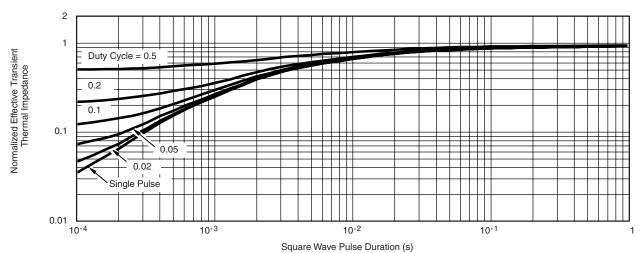
Normalized Thermal Transient Impedance, Junction-to-Case
