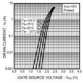
Fig.4 Typical Transfer Characteristics
