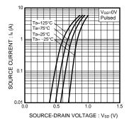
Fig.6 Source Current vs. Source-Drain Voltage
