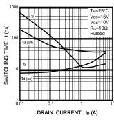
Fig.2 Switching Characteristics
