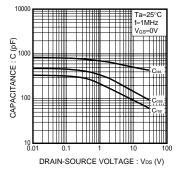
Fig.1 Typical Capacitance vs. Drain-Source Voltage
