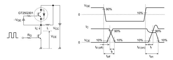
Note2: Switching loss measurement waveforms
