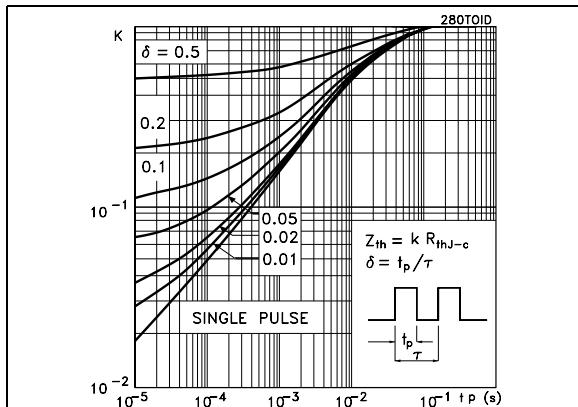
**Figure 15. Thermal impedance for TO-220FP**
