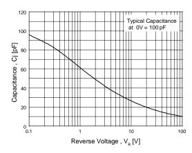
Figure 3. Typical Junction Capacitance
