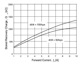
Figure 5. Typical Stored Charge vs. Forward Current
