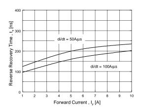
Figure 4. Typical Reverse Recovery Time vs. Forward Current
