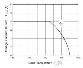
Figure 6. Forward Current Derating Curve
