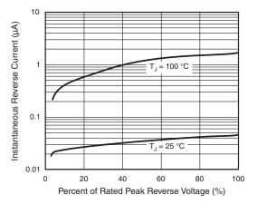
Fig. 4 - Typical Reverse Characteristics
