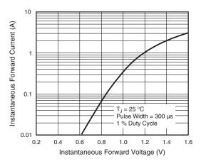
Fig. 3 - Typical Instantaneous Forward Characteristics
