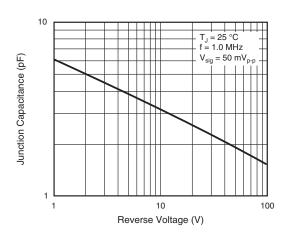
Fig. 5 - Typical Junction Capacitance
