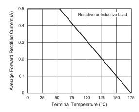
Fig. 1 - Forward Current Derating Curve
