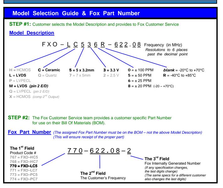
This example, FXO-LC536R-622.08 = LVDS Output, Ceramic, 5 x 3.2mm Package, 3.3V, ±25 PPM Stability, -40 to +85°C Temperature Range, at 622.08 MHz
