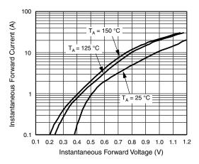
Figure 3. Typical Instantaneous Forward Characteristics
