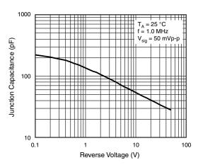
Figure 5. Typical Junction Capacitance
