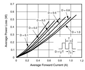
Figure 2. Forward Power Loss Characteristics
