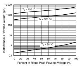
Figure 4. Typical Reverse Leakage Characteristics
