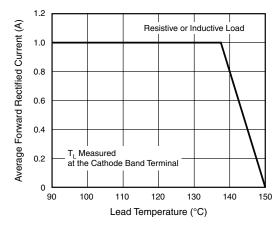
Figure 1. Maximum Forward Current Derating Curve
