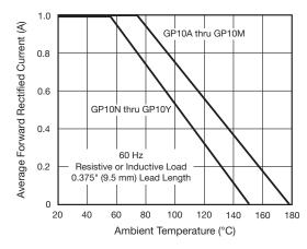
Fig. 1 - Forward Current Derating Curve
