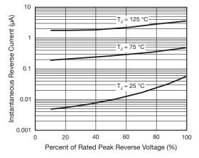
Fig. 4 - Typical Reverse Characteristics
