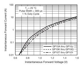
Fig. 3 - Typical Instantaneous Forward Characteristics
