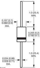
• Lead diameter is  $\frac{0.020 (0.5_{-})}{0.023 (0.58)}$ 0.026 (0.66) for suffix "E" part numbers
