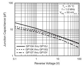
Fig. 6 - Typical Junction Capacitance
