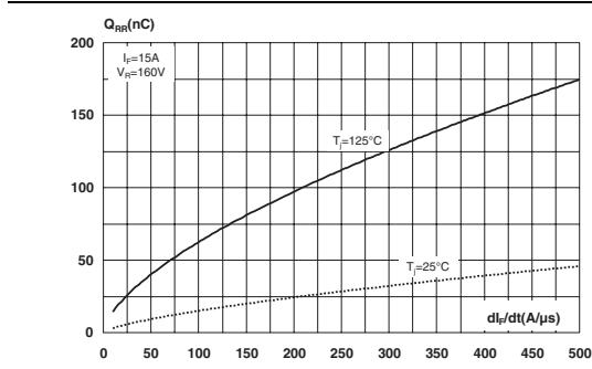
**Figure 8. Reverse recovery time versus dI\_F/dt (typical values)**
