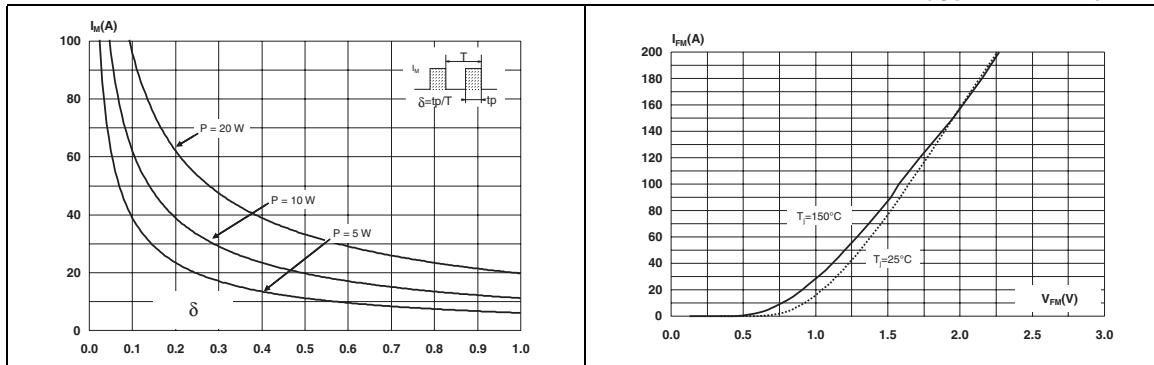
**Figure 3. Forward voltage drop versus forward current (maximum values)****Figure 4. Relative variation of thermal impedance, junction to case, versus pulse duration (TO-220AC)**
