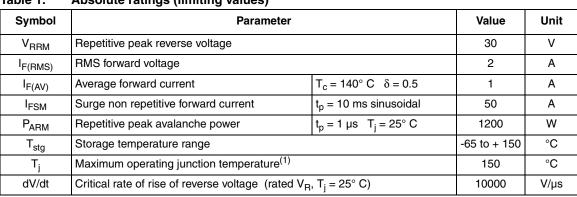
1.  $\frac{dPtot}{dTj} < \frac{1}{Rth(j-a)}$  condition to avoid thermal runaway for a diode on its own heatsink
