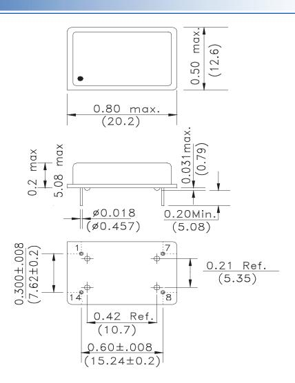
The height of the package vary depending on the frequency >100MHz. Please contact ABRACON for the height information for F>100MHz.
