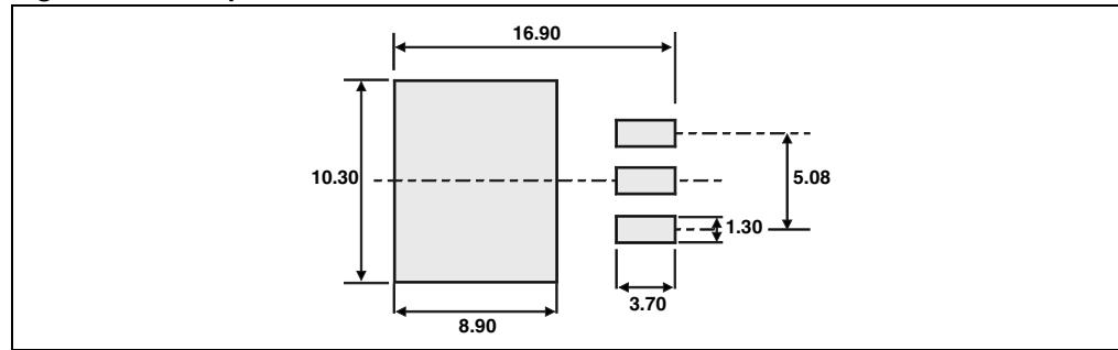
Figure 14. Package dimensions TO-220AB
