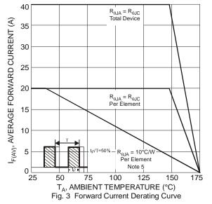
Notes: 5. Black Aluminium Heatsink; length 37mm, width 15mm, height 50mm.
