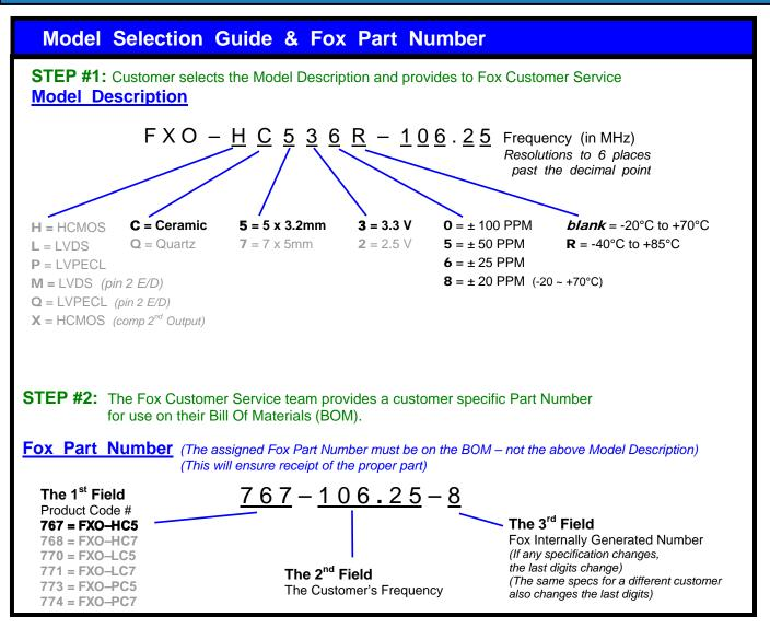
This example, FXO-HC536R-106.25 = HCMOS Output, Ceramic 5 x 3.2mm Package, 3.3V, ±25 PPM Stability, -40 to +85°C Temperature Range, at 106.25 MHz
