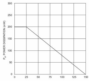
$T_A$ , AMBIENT TEMPERATURE (°C) Fig. 4 Power Derating Curve, Note 1
