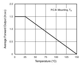
Figure 1. Derating Curve Output Rectified Current
