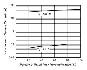
Figure 4. Typical Reverse Characteristics Per Diode
