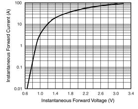
Figure 3. Typical Forward Characteristics Per Diode
