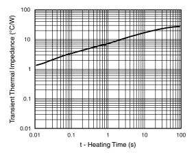
Figure 6. Typical Transient Thermal Impedance
