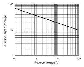
Figure 5. Typical Junction Capacitance Per Diode
