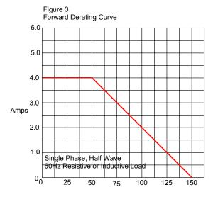
Average Forward Rectified Current - Amperes versus Case Temperature -  $^{\circ}$ C
