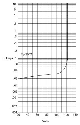
Instantaneous Reverse Leakage Current - MicroAmperesersus Percent Of Rated Peak Reverse Voltage - Volts
