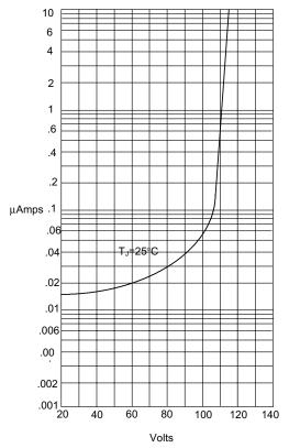
Instantaneous Reverse Leakage Current - MicroAmperewersus Percent Of Rated Peak Reverse Voltage - Volts
