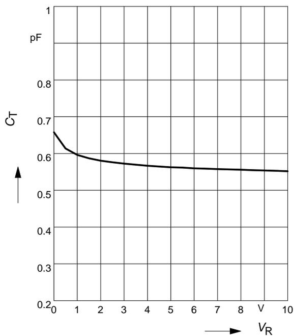
**Diode capacitance  $C_T = f(V_R)$**
