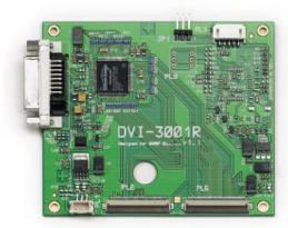
The DVI-3001/2/3/XR is a family of all digital interfaces for Sharp TFT LCD panels to give the best picture performance possible. No analogue conversion is used to possibly degrade the image displayed. The DVI-3001/2/3/XR allows for interfacing between any DVI compatible graphics interface/card and a Sharp TFT LCD panel. All settings and panel specific data is pre-programmed for true Plug&Play function when used with Windows NT/98/95.
