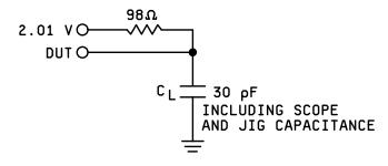
$t_{DF}$  is tested with  $C_L = 5$  pF.
