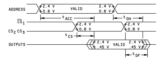
FIGURE 3. AC read timing diagram.
