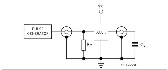
$C_L$  = 50pF or equivalent (includes jig and probe capacitance)  $R_T$  =  $Z_{OUT}$  of pulse generator (typically 50 $\Omega$ )
