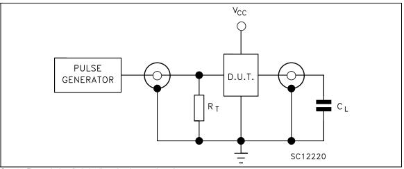
$C_L$  = 50pF or equivalent (includes jig and probe capacitance)  $R_T$  =  $Z_{OUT}$  of pulse generator (typically 50Ω)
