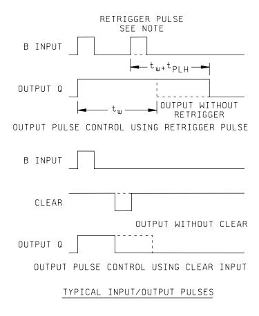
NOTE: Retrigger pulse must not start before 0.22 C<sub>X</sub> (in picofarads) nanoseconds after previous trigger pulse.
