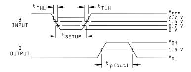
1. The pulse generator has the following characteristics:  $V_{gen}$  = 3.0 V,  $t_{THL} \le$  10 ns,  $t_{TLH} <$  10 ns,  $t_{SETUP}$  = 60 ns,  $Z_{OUT} \approx 50 \ \Omega$ , and PRR is as follows:
