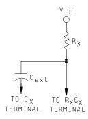
These circuits are fully compatible with most TTL or DTL families. Inputs are diode-clamped to minimize reflections due to transmission-line effects, which simplifies design. Typical power dissipation per one shot is 115 milliwatts; typical average propagation delay time to the Q output is 21 nanoseconds.
