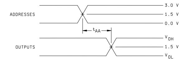
FIGURE 3. Switching time test circuits and waveforms - Continued.
