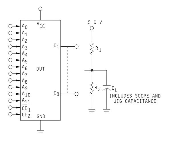
Note:  $R_1 = 270\Omega$  and  $R_2 = 600\Omega$   $C_L = 50 \ pF$
