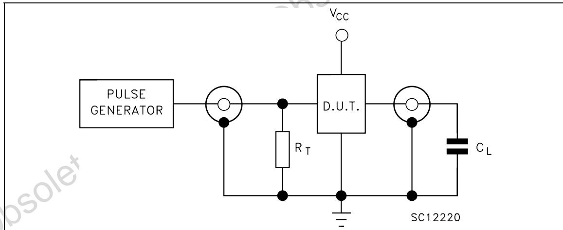
$C_L = 50\text{pF}/150\text{pF}$  or equivalent (includes jig and probe capacitance)
