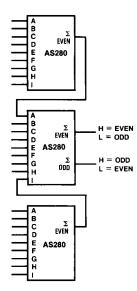
FIGURE 1. 25-Line Parity/Generator Checker
