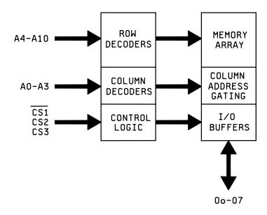
FIGURE 3. Block diagram.
