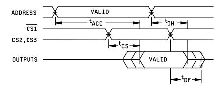
FIGURE 5. AC read timing diagram.
