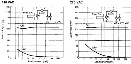
Note: When the current rating of the load is less than 10 mA, false operation may occur. This is normal, and the problem can be solved by installing a bleeder resistor in parallel with the load. Use the formulas given here to calculate the power rating and value of the resistor.
