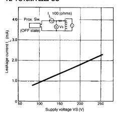
Note: Even when the proximity sensor is in the OFF state, a very small amount of current flows to operate the internal circuit of the sensor. Because of this leakage current, a small voltage is generated in the load, which may occasionally result in improper resetting of the load. Before using the proximity sensor, confirm that this voltage is less than the release voltage value of the load.
