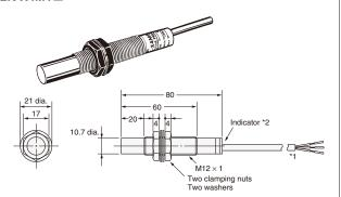
\*1. E Models: 4-dia. vinyl-insulated round cable with 3 conductors (Conductor cross section: 0.2 mm², Insulator diameter: 1.2 mm), Standard length: 2 m Y Models: 4-dia. vinyl-insulated round cable with 2 conductors (Conductor cross section: 0.3 mm², Insulator diameter: 1.3 mm), Standard length: 2 m 2. E Models: Detection indicator (red) Y Models: Operation indicator (red)
