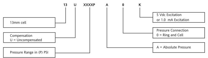
For example: **Part #13U 3000PA0K** = 13 mm Cell, Uncompensated, 3000 psi, Absolute, Ring pressure connection with 5 Vdc excitation.
