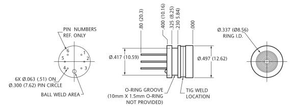
**Note:** Non-concentricity effects at the diaphragm weld area may cause runout of up to  $\pm 0.006$  in between the upper and lower portions of the sensor body. (It is recommended to use a counter bore to mate with this device to allow for this non-concentricity).
