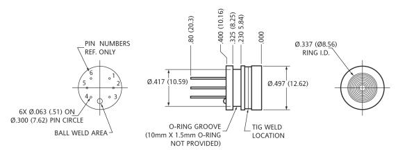
**Note:** Non-concentricity effects at the diaphragm weld area may cause runout of up to  $\pm 0.006$  in between the upper and lower portions of the sensor body. (It is recommended to use a counter bore to mate with this device to allow for this non-concentricity).
