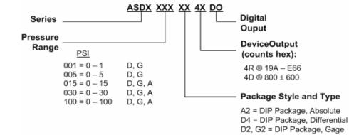
For example: Part #ASDX015A24RD0 = ASDX series, 15 psi absolute, A2 Package, 19A - E66 counts output , digital output
