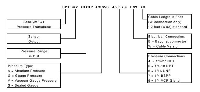
For example: Part #SPTmV0100PA4W02 = SPT mV Sensor, 100 psi, Absolute, 1/8NPT Port, with a 2 feet cable (pigtail) electrical connection.
