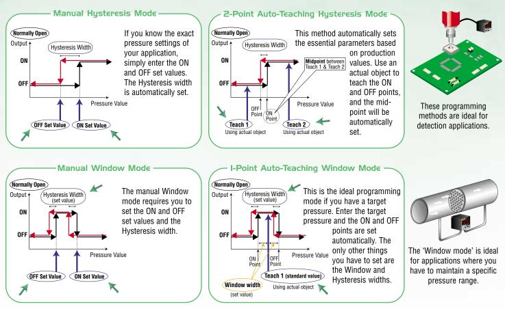
NOTE: The above charts show a 'Normally Open' configuration. Reverse them for a 'Normally Closed' configuration. Downloaded from Elcodis.com electronic components distributor
