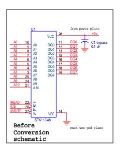
In this conversion, old bypass capacitor C1 is moved from +5v on pin 28 to pin 1. It is essential that pin 28 be left OPEN and system power (+5v) is now connected to pin 1 (VCAP). The new signal /HSB is left open and unused. This will configure the STK12C68 into a non-autostore part. The storage capacitor is not needed since autostores are deselected. Software stores use system power to complete commanded stores. The extra address pins (A11 and A12) are tied inactive to ground.
