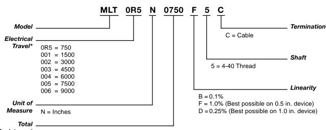
Note: Not all combinations are available. Minimum quantity orders apply. Contact the factory for more details. \* Note: The *Electrical Travel* correlates to the *Total Resistance (Ohms)*.
