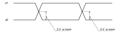
**Remark** Adjust cross point of  $\phi$ 1,  $\phi$ 2 by  $\phi$ 1,  $\phi$ 2 pin external input resistors.
