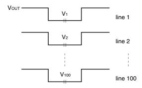
This is measured by the DC level sampling of only the signal level, not by CDS (Correlated Double Sampling).
