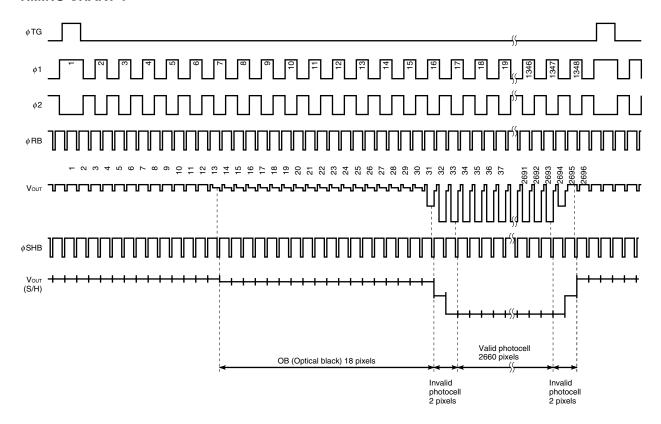
**Remark** Vout = Output when  $\phi$ SHB is not in used (When  $\phi$ SHB is not in used, connect  $\phi$ SHB pin to GND). Vout (S/H) = Output when  $\phi$ SHB is in used.
