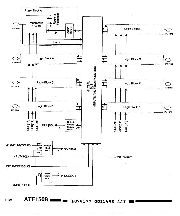
The ATF1508 macrocell is flexible enough to support highly complex logic functions operating at high speed. The macrocell consists of five sections: product terms and product term select multiplexer; OR/XOR/CASCADE logic; a flip-flop; output select and enable; and logic array inputs.
