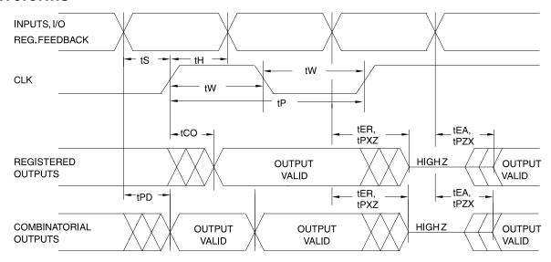
Note: 1. Timing measurement reference is 1.5V. Input AC driving levels are 0.0V and 3.0V, unless otherwise specified.
