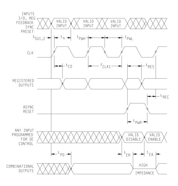
FIGURE 4. Switching waveforms.
