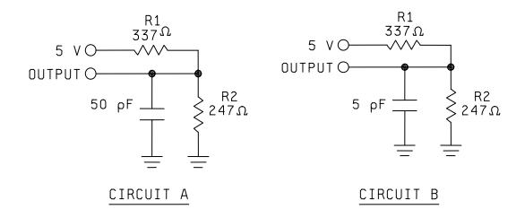
FIGURE 3. Output load circuit.
