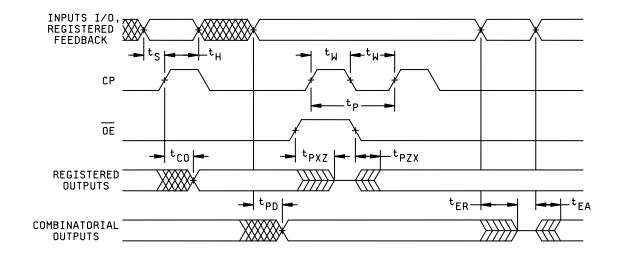
FIGURE 4. Switching waveforms.
