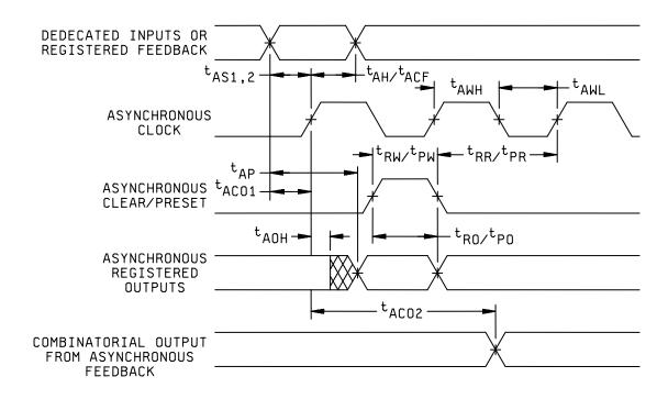
FIGURE 5. <u>Switching waveforms</u> - Continued.
