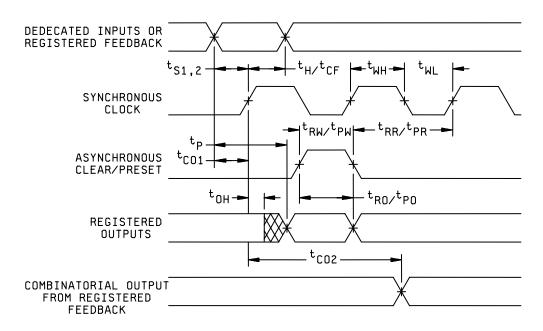
FIGURE 5. Switching waveforms.
