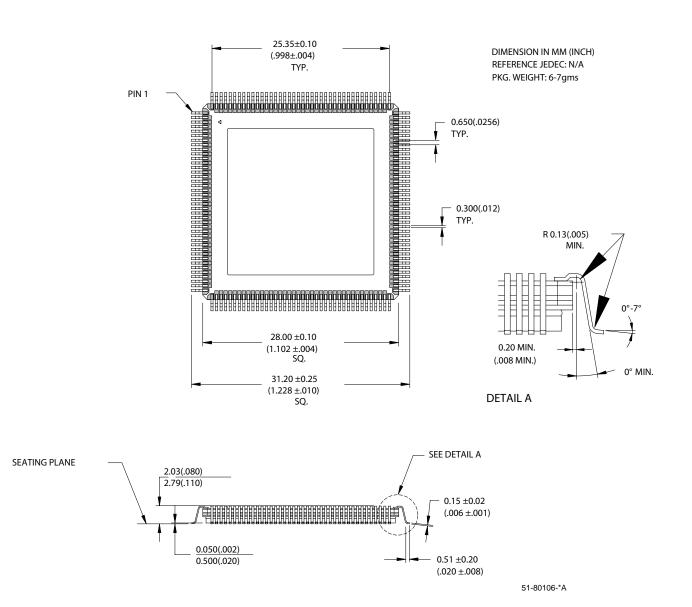
160-Lead Ceramic Quad Flatpack (Cavity Up) U162
