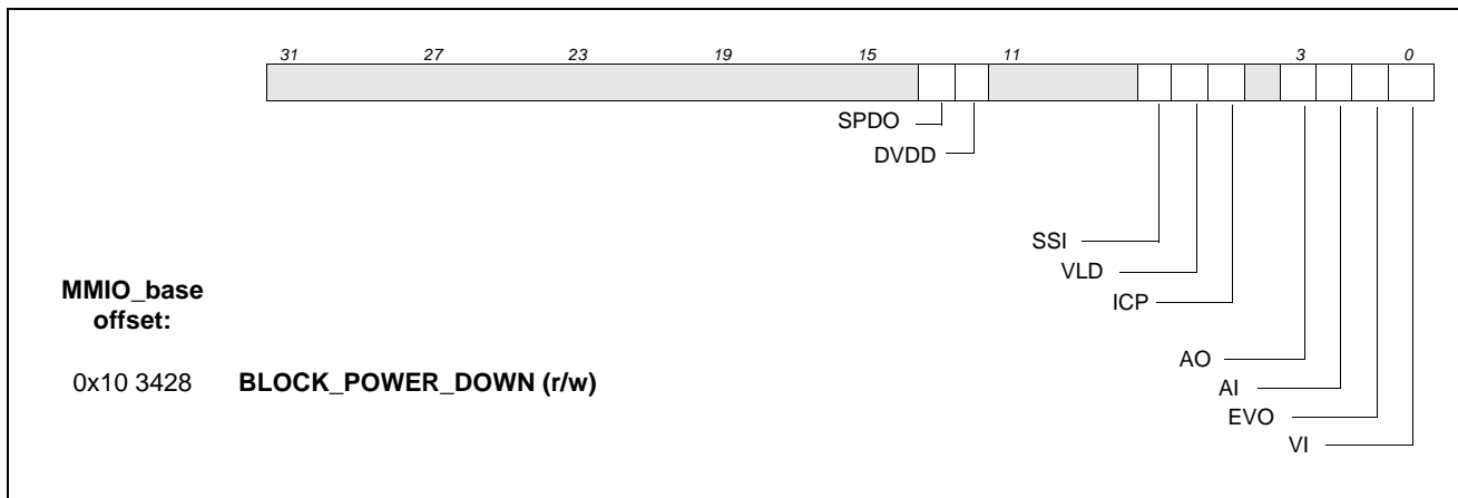
Figure 21-1. Power down register BLOCK_POWER_DOWN
